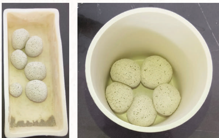
Synthetic slag prepared using aluminium dross and other industrial wastes
