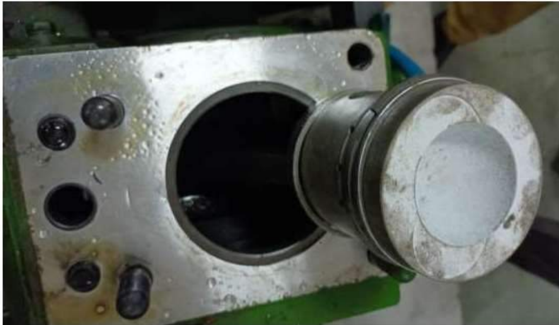
Nano ceramic coated Piston (NiCrAlY/YSZ) mounted on diesel engine
