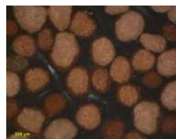
Sphericity & Roundness of Proppant
