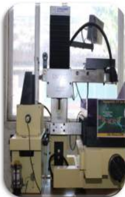
Computer Numerically Controlled Wire Cut Electrical Discharge Machining (CNC Wirecut EDM)
